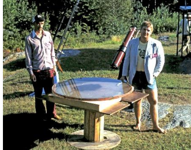
John Briggs with the flat used for testing the 36" Lick lens
