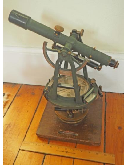
A typical early 20 th century transit. My Buff & Buff transit with horizontal and vertical scales reading to one minute on the verniers.
