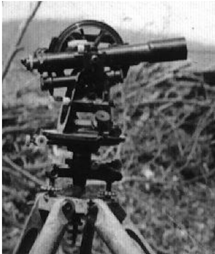
What instrument is this? I believe this is one of the two Berger theodolites with 4-inch circles described in the report of the Fiala Ziegler Polar Expedition (Porter used one of these on the Alaska expedition). See the stencil on the tripod leg. Photo stm0118 from STM Photo Archive.
