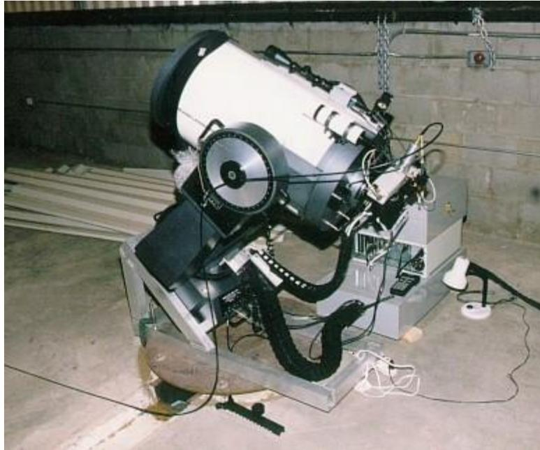
The image above shows their 16 inch telescope with custom-made fiber optic cable (running along the ground to the left of the image). This fiber is connected to a large, table mounted spectrometer using this design:
