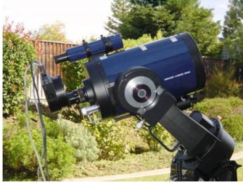
That is an 8 inch Schmidt-Cassegrain telescope with a 765x510 pixel CCD camera - total cost is about \$4000.00 - not bad! The light curve from this telescope is below:
