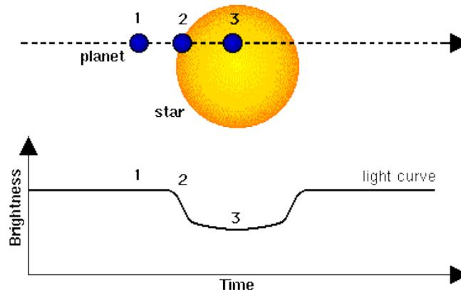
As a planet passes over the portion of the star facing us, the light curve of the star drops for a time. As the planet passes through, the light curve returns to normal. The image below shows a typical setup for an amateur to capture images of the transit:
