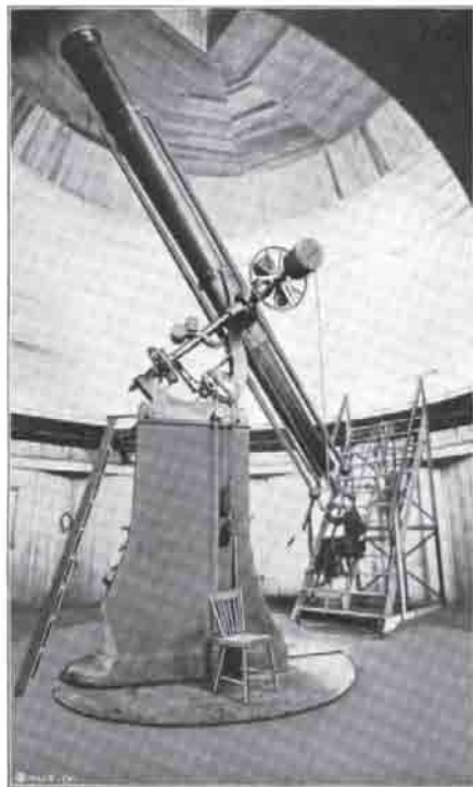
THE 18½-INCH CLARK TELESCOPE OF THE OLD UNIVERSITY OF CHICAGO (DEARBORN OBSERVATORY)
