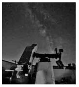
tween 1989 and 1995. It houses a unique instrument—a 13" f/10 Schupmann telescope mounted on a massive computer controlled alt-az mounting. For a time it was the largest operating Schupmann in the world. This design, which combines reflective and refractive elements, yields a coma-free and essentially apochromatic image, and is ideal for planetary observation. The Schupmann is operated during Convention. Photo by Dennis di Cicco.
