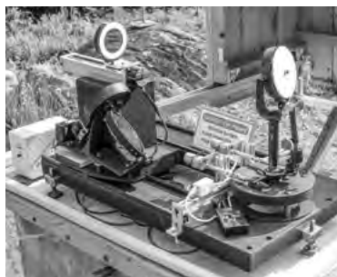
The coelostat and objective lens (top left), with new motorized controls that replace the old mechanical links. Photo: Sal LaRicca
