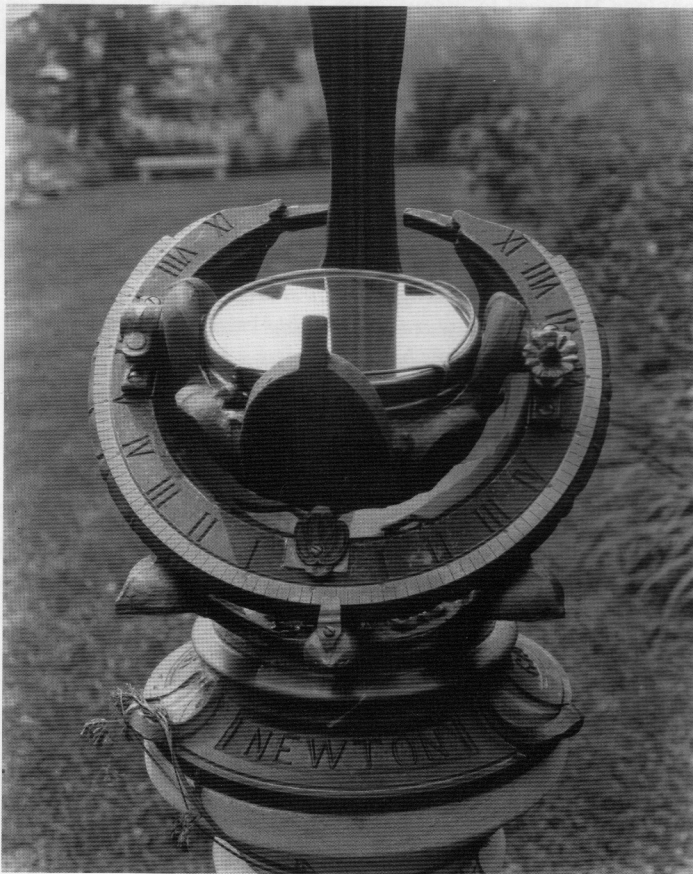
Figure 2: A close-up showing details of the base, split-ring hour circle, and bowl holding the mirror. Date unknown, early 1920s.
