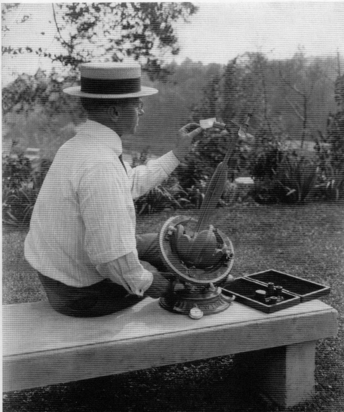
Figure 1: Russell W. Porter demonstrating how his Garden Telescope may be used as a sundial by directing the sun's image onto a card and reading the sun's hour angle from the hour circle. Date unknown, early 1920s.
