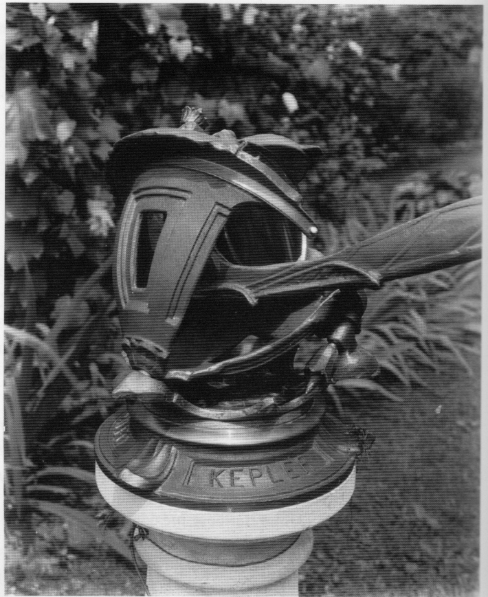
Figure 3: A close up showing details of the base, bell, and one of the knobs for turning the telescope in right ascension (seen on the right). Date unknown, early 1920s.
