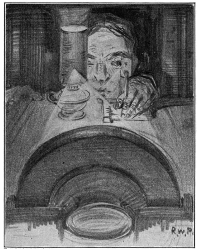
FIGURE 3: THE FOUCAULT, KNIFE-EDGE TEST With a lamp and razor blade, imperfections of the order of a millionth of an inch can be detected
