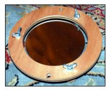
The mirror cell has two main parts, the ring (one of the four rings) and the mirror back.
