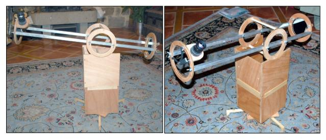
During my last trip in the US, I was able to pick a 114mm/25.4mm primary/secondary mirror pair for 18\$ (Telescope warehouse on eBay). After a lot of back and forth, I decided to make a travel telescope out of it.
